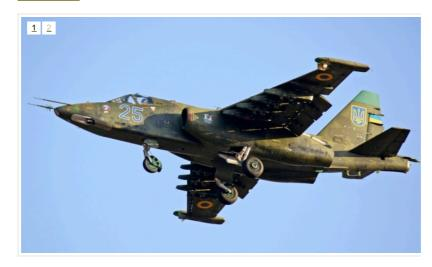
Su-25 is designed for direct aviation support of the Army, destruction of small-size moving and fixed objects under conditions of visibility at the forefront in tactical and nearest operative depth.
