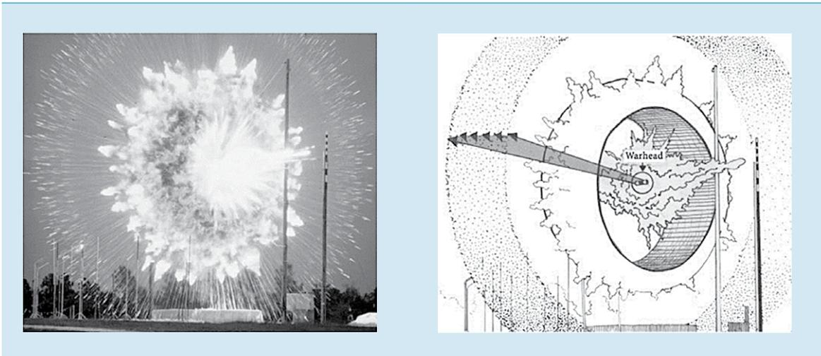
Figure 54: Fragmentation pattern of a stationary, horizontal high-explosive fragmentation warhead detonation. (Source: *The Fundamentals of Aircraft Combat Survivability Analysis and Design*<sup>19</sup>, Robert E. Ball, reprinted by permission of the American Institute of Aeronautics and Astronautics, Inc.)
