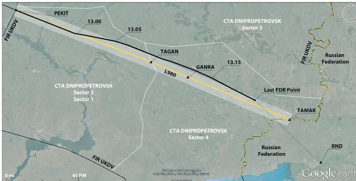
Figure 3: Route of flight MH17 across the eastern part of Ukraine. The light grey shading shows the area that is 5 NM left and right of the centreline of airway L980. The black line shows flight MH17 deviating from airway L980 between air navigation waypoints PEKIT and TAGAN. (Source: Google, Landstat)
