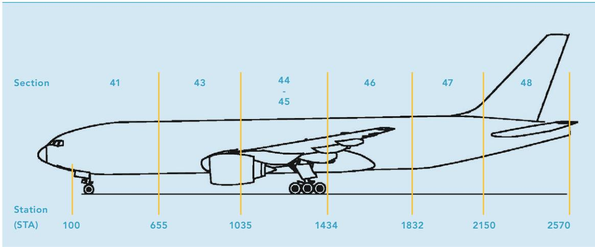
Figure 90: Schematic diagram of Boeing 777 Sections and Stations. (Source: Dutch Safety Board)
