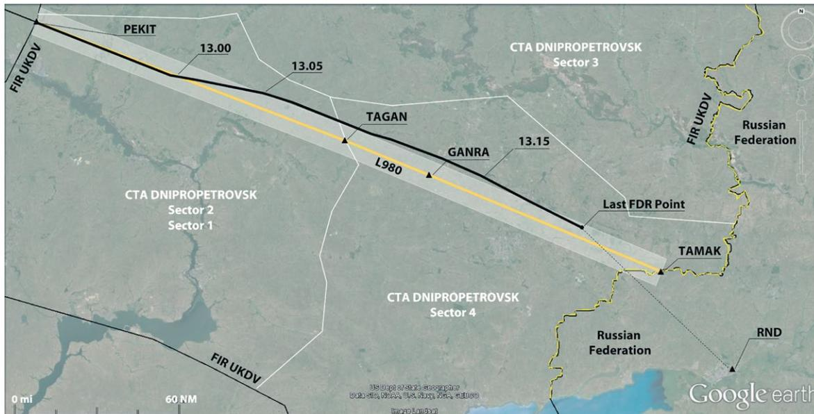
Figure 85: Image of the Dnipropetrovsk FIR (UKDV), CTA 1 and 4, and the flown (black line) and intended (dotted black line) route of flight MH17. The yellow line represents the centre of airway L980. (Source: UksATSE and Google, Landstat)
