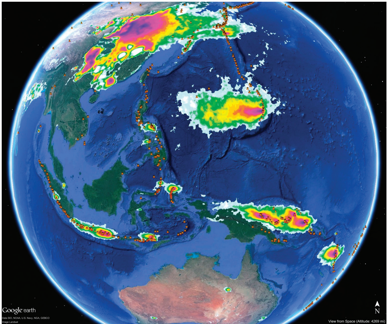
FIGURE 4.2 Map of anthropogenic and volcanic \text{SO}_2 sources in East Asia and the western Pacific region based on Ozone Monitoring Instrument satellite data collected in 2005–2007. \text{SO}_2 detected over East Asia is mostly anthropogenic \text{SO}_2 emissions from China; the other \text{SO}_2 sources are mostly due to passive volcanic degassing. Significant volcanic \text{SO}_2 emissions can be seen in Japan, the Mariana Islands, the Philippines, Indonesia, Papua New Guinea, and Vanuatu. SOURCE: Based on data from Fioletov et al. (2016).
