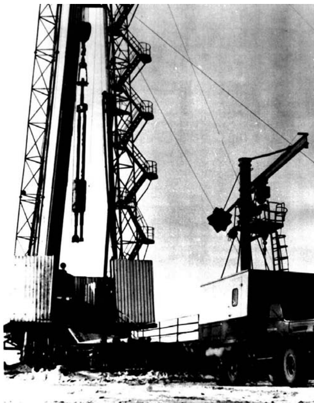
Figure 29. Drill rig, of the type used for drilling the nuclear test emplacement borehole. Normally, the emplacement borehole has a diameter of ~900 millimeters, and was drilled to depths ranging from 200 to about 1000 meters. The rig shown was that used to drill the hole for the Soviet nuclear test of the US-USSR Joint Verification Experiment, conducted at the Balapan test site in 1988.
